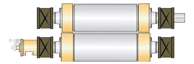
The quick adjustment system we offer for sets of top-to-flat rolls is a patented system allowing to modify the required embossing nip within a few seconds. It makes e.g. a switch from 3- to 2-ply material and vice versa possible and allows to make the readjustment generally required.
